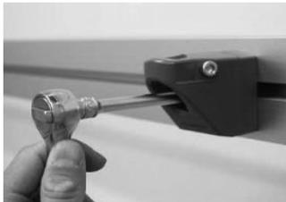
Attach the bracket onto conveyor beam and tighten with long wrench.
