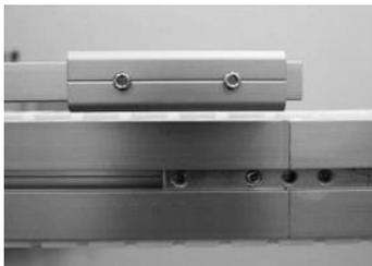
First, fully slot the guide rail sleeve into either one of the guide rail profile that you are going to join.
